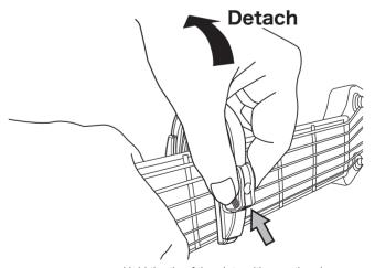
Hold the tip of the plate with your thumb and index finger. Pull it up to slide carefully.
